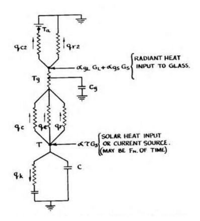
Figure 1.2: A thermal of a single basin solar still. Source: Dunkle (1961)
